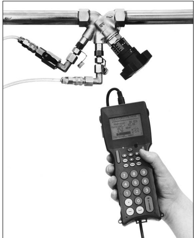
Flow-meter "OV-DMC 2", item no. 106 91 77 with "Hydrocontrol R"
